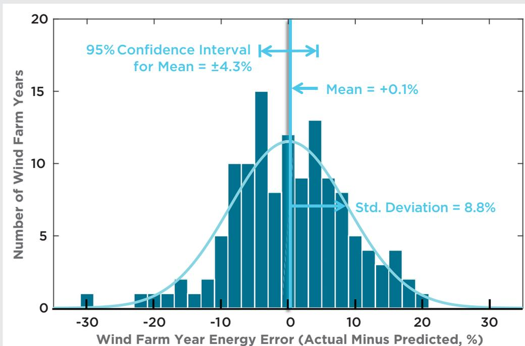
*Histogram of wind farm year energy errors (1-year actual minus long-term predicted, %). The vertical line shows the mean bias error (+0.1%). The bell curve shows the fitted normal distribution using the mean bias and standard deviation of errors. The interval at the top indicates the 95% confidence interval on the mean bias error.*
